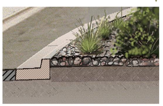
The curb for the islands has a 24 inch gutter pan. Finished grade is about 4 inches below the top of the curb with cobble mulch.
