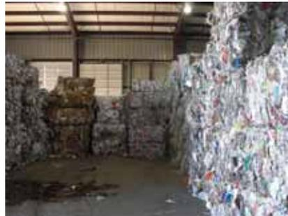
Separated material is baled and stacked in preparation for shipment to processors in other states.
