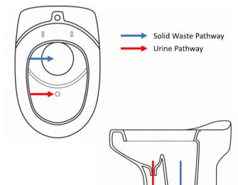
The proposed design would be a common portable toilet retrofitted with a urine diverting seat insert, as shown above
